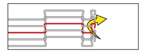
• Connect the splice strand edge hook to the near side loop edge using pliers hooking up under the near edge strand.
